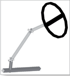
Steering linkage with 3D representation of shaft and joints, including the resulting nonlinear steering wheel-to-rack ratio.
